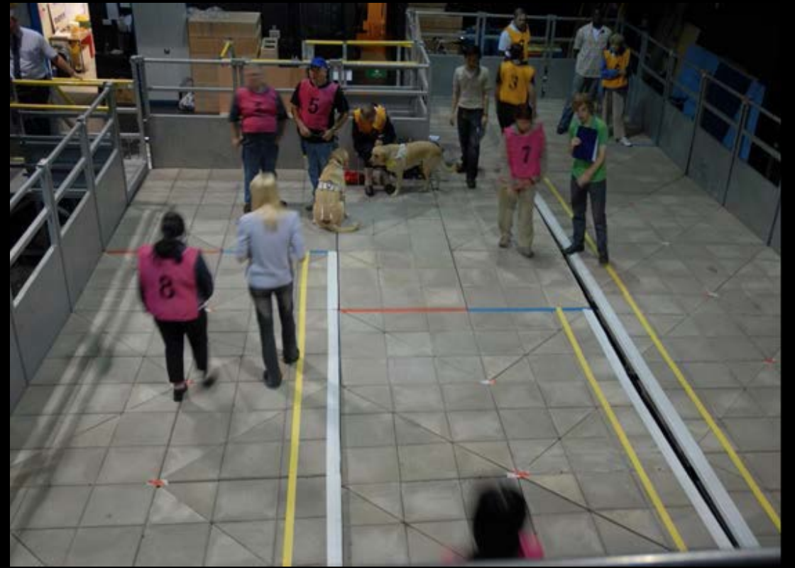
Experiment about platform gradients for people with vision challenges and their assistance dogs
